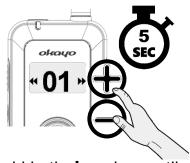
Press and hold both  $\underline{+}$  and  $\underline{-}$  until above display shows up. Select an assigned channel via  $\underline{+}$  or  $\underline{-}$  and confirm/leave with a press of  $\vdots$ .
